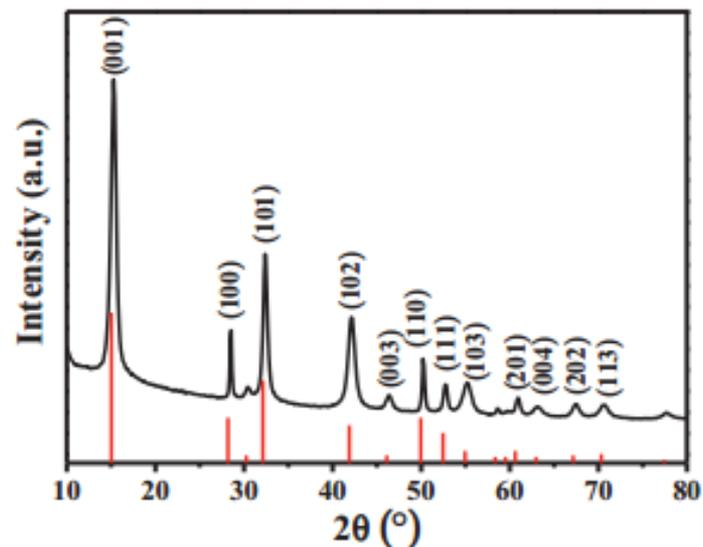
Fig. 1. XRD patterns of SnS<sub>2</sub>-200-10.5 (the bottom of the image indicates the JCPDS data (JCPDS: 23-0677) for SnS<sub>2</sub>).
