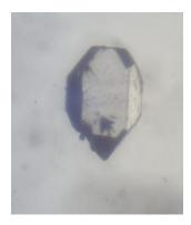
This is a photo of an example of a good crystal. The crystal is of good crystal quality because it has a clear face.
