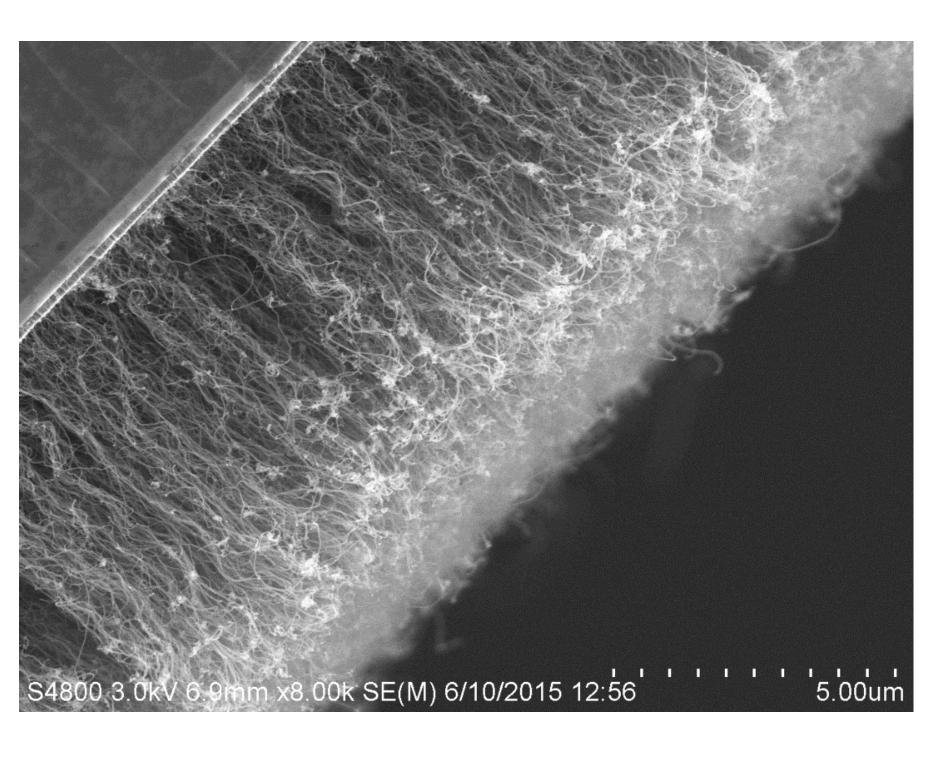
Some of the pore-structure properties of carbon nanotube forests are thought to be linked to their area packing density. Previous experiments have shown some correlation between the temperature at which the carbon nanotubes were grown and the resulting area density.
