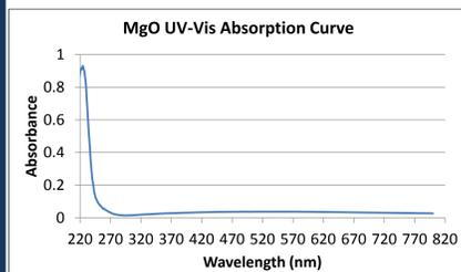
Figure 4. Based on the UV-Vis curve, it is clear that MgO is transparent to visible light as desired.
