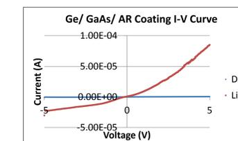
Figure 9. Ge/ GaAs with AR coating I-V curve. A clear improvement is seen from the AR coating. There is a non-linearity as desired. A rectifying effect is observed.
