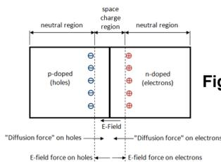
Figure 1. Schematic of a p-n junction.<sup>1</sup>
