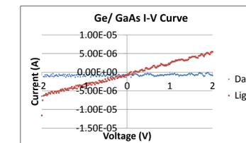
Figure 8. Ge/ GaAs I-V curve. A solar effect is clearly seen upon comparison between light and dark curves. Again, the curve is quite linear.
