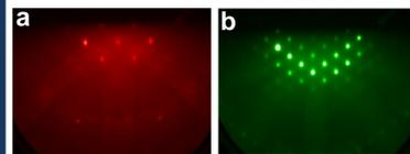
Figure 3. Example RHEED Images of GaAs (2a) and Ge (2b). Both are epitaxial.
