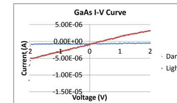
Figure 6. GaAs I-V curve. A solar effect is clearly seen upon comparison between light and dark curves. However, the light curve is quite linear. No rectifying effect is observed.
