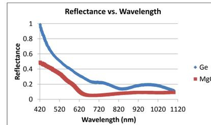
Figure 5. MgO serves as a great AR coating-especially at lower wavelengths.
