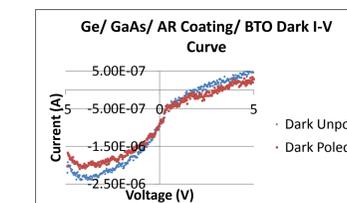
Figure 10. With BTO dark I-V curve. The poled BTO reduced the dark current as desired.
