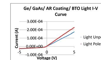
Figure 11. With BTO light I-V curve. The poled BTO increased the light current and non-linearity as desired.
