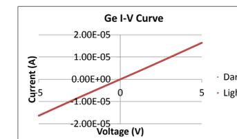
Figure 7. Ge I-V curve. No solar effect is observed. The light and dark curves are the same in this case.
