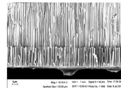
Figure 5: SEM image of nanowires grown on Ag
