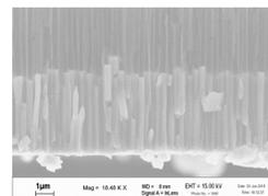
Figure 4: SEM image of nanowires grown on Cu
