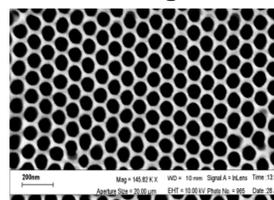
Figure 2: SEM image of lab-grade AAO template
