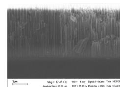
Figure 6: SEM image of nanowires grown on Al
