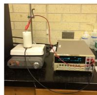
Figure 1: Electrodeposition setup
