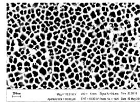
Figure 3: SEM image of commercial-grade AAO template
