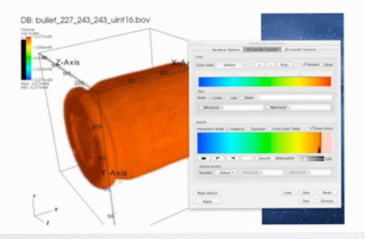
Second, show the low-intensity numbers. Problem: the propellant grains are supposed to be the highest intensity voxels. The numbers above 215 were converted to negative values.
