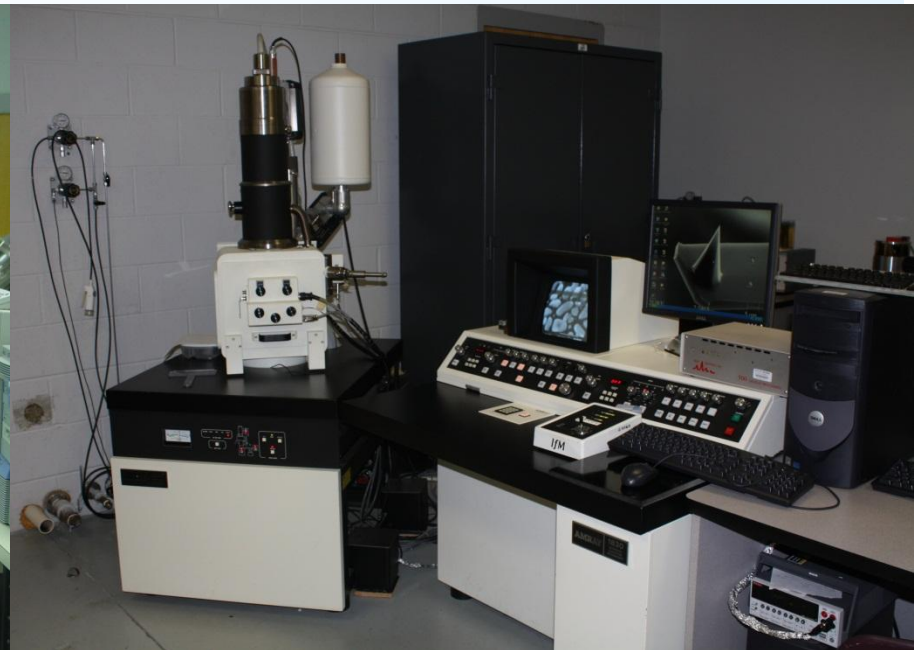
Amray 1830 SEM Thermionic Emission
