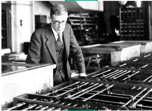
Bush Differential Analyzer - www.britannica.com
